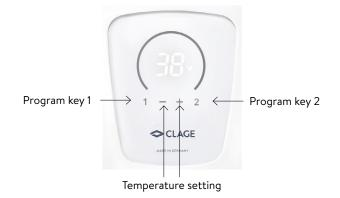
The DCX Next L is operated via a LED display with sensor keys. The two programming keys are preset to 38 °C and 42 °C and can be individually adjusted. Unit parameters can be read out and set via a service menu.
